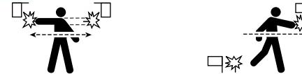
Horizontal waving of white flag, light or flare. Putting one flag, light or flare on ground and moving off with a second indicates direction of safer landing.
